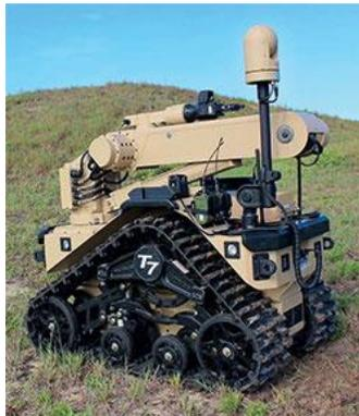
The completed solution from Doodle Labs was successfully integrated into the T7. In field tests, the system was able to double Harris' 100 meter NLOS requirement and achieve operation from 200 meters away through a building.
