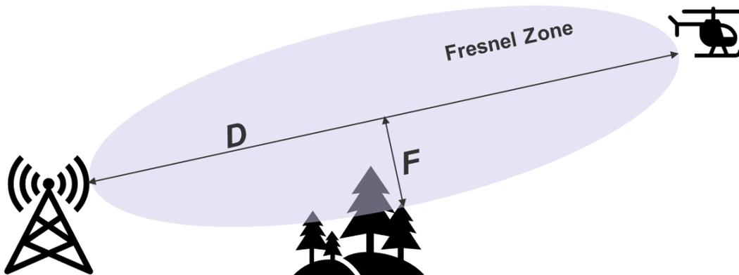
Due to dispersion, the Fresnel zone size increases as the signals travel further out. Mid-point of the link has the biggest Fresnel zone. Another important factor is the frequency. Lower
