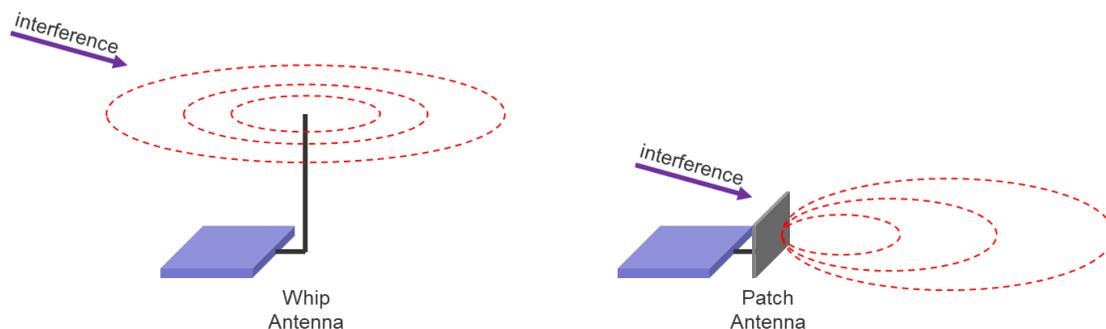
The second example is of a directional antenna in both the elevation and azimuth. By focusing the RF power in a smaller beam width, provides important benefits like higher gain to achieve longer range. They also help avoid interference originating outside of the link path. Looking at the diagram above, the directional antenna could get a significantly better link quality because it cannot “see” the interference coming from the back of the antenna.
