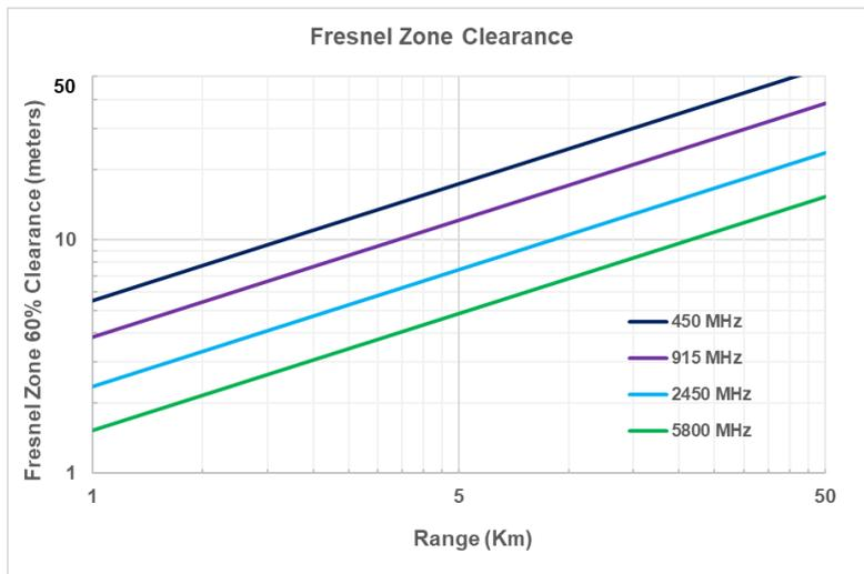
When designing the RF link for mobile nodes, it is important to consider the potential Fresnel zone obstruction at all locations.
