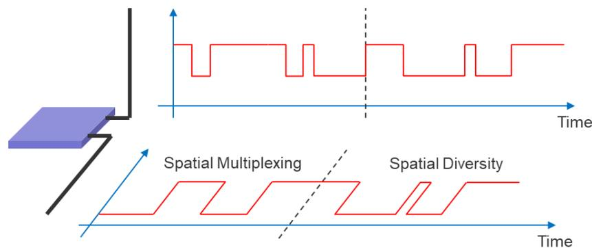
In spatial-multiplexing, two different streams of data are sent to the two antennas resulting in double the throughput. In order not to interfere with each other in a line-of-sight (LoS) link, the antennas should be oppositely polarized. In a non-LoS link, it is not necessary for the antennas to be oppositely polarized as the radios make use of multipath propagation to combine the data streams.
